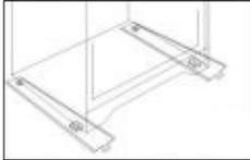
Position the sliders parallel on the floor in a position to be underneath the legs of the appliance.
